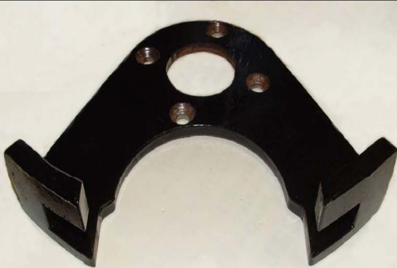
Backing plate for Toro / Eldorado type calipers, fork design similar to drop forged front knuckle
