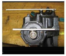
To be certain that the steering wheel remains horizontal, it should be locked in place with a long object and tie wraps (do not use the ignition switch key lock). Also, at the same time, the wheels should be pointing straight ahead as you drove it straight into position.
