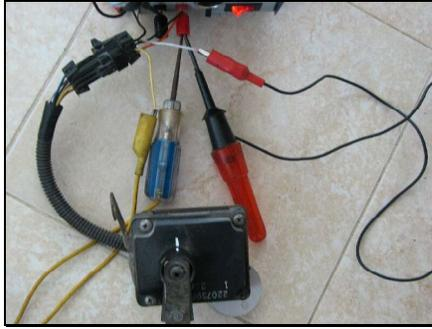
***Slide comes after 25***The circuit is cancelled if the lever is moved to the neutral position.
