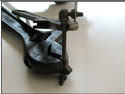
The orientation of the stud balls on the link can easily be done by using to wrenches on the flats of the ends to rotate them into position.
