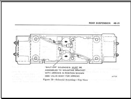
In my opinion these arrow are 'WRONG'. They should point toward the normal lowest pressure. The internal spring must keep the valve closed if mounted in this orientation. Over the years they tend to leak. If mounted the opposite direction then the pressure keeps the valve closed.
