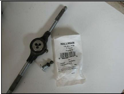
Rethread the stud ball to 1/4 x 20 threads to match those on the 'T nut'.
