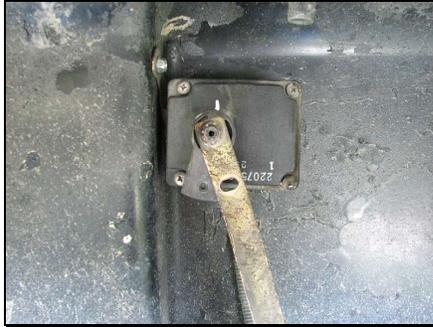
Mount the sensor in the center recess of the wheel well. It should be as close to the top and back wall as possible so that it is out of the way and is not obstructed in movement.
