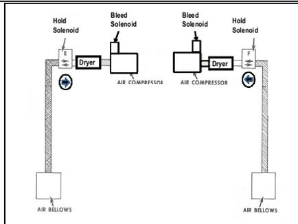
**Air schematic of Electro Level II- Minimal hoses** from compressor to Air Bags
