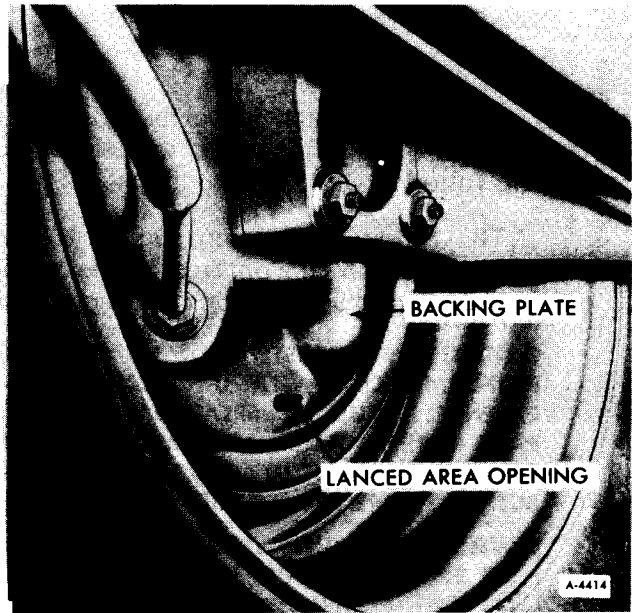
Figure 3—Lanced Area in Backing Plate
