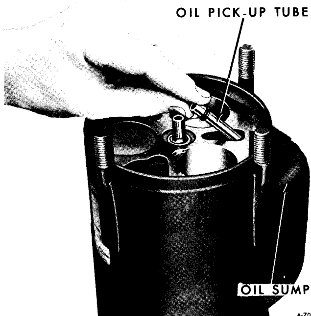
Figure 133—Installing Oil Pick-Up Tube
