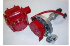
distributor cap and mark its post with masking tape. Set the cap back on the distributor and put a small piece of tape (marked as tape #2) on the distributor housing directly below your #1 plug wire terminal (post). Next, put a third tape tag (#3) on the block 'directly' in line below your #2 tape. Now tip the cap back and see if the rotor tip is pointing to the #1 post (which is marked with the #3 tape on the base).
