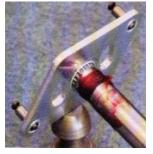
Take each weight off and wire its spring to it (so they are married). Remove the two clips from the pins that stick up through the **center cam**. Remove it and the pole piece (with the 8 teeth) will slide down and off the shaft. Clean up and re-grease the top grease groove on the shaft. Re-assemble. Put on the center cam **numbers facing down (repeat numbers down)**.
