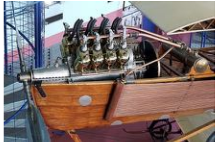
An Antoinette mechanically fuel-injected V8 aviation engine of 1909, mounted in a preserved Antoinette VII monoplane aircraft.
