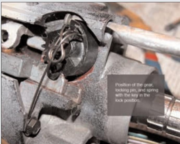
Reinstall the tilt spring. Reverse the procedure for removal.
