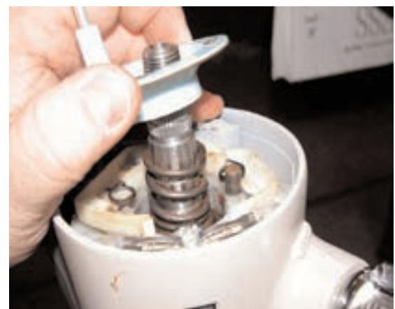
**Remove the blinker arm and the three screws that hold in the blinker switch in place. Remove the spring and the spring seat.**
