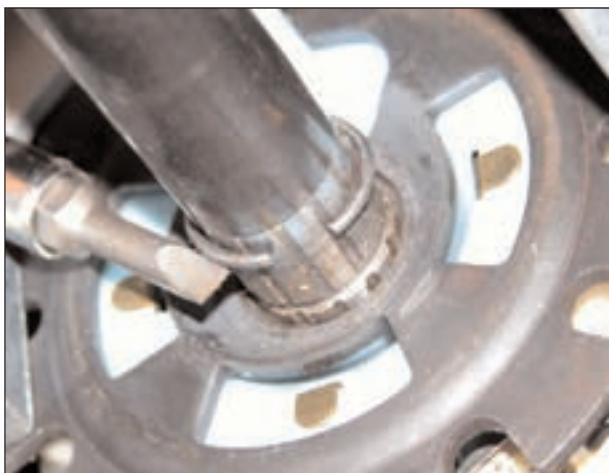
Then remove the Spring compressor, and take off the locking plate, and the flasher return cam.
