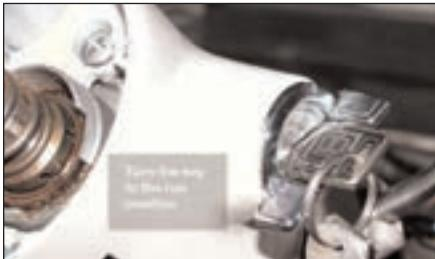
Put the key in the run position. Use a screw driver to push the tab up. Then slide out the key cylinder.
