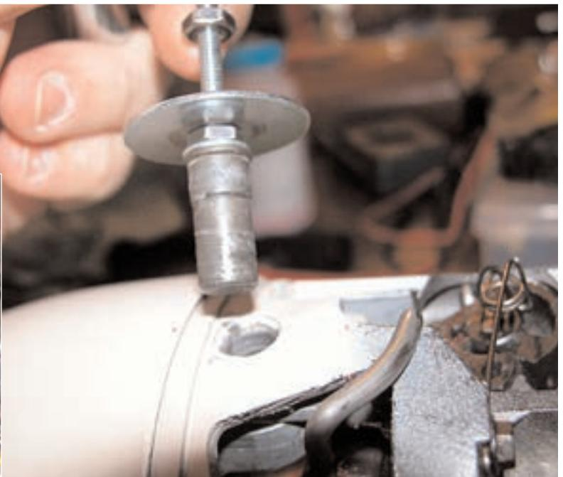
**Replace the tilt lever.** Pull the lever to release the lock and pull the upper tilt block away from the lower part of the column.
