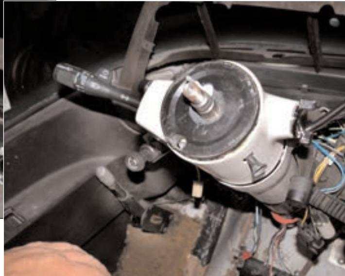
Remove turn signal handle, the emergency flasher button, and the tilt handle. On a GMC column you will have to wait to remove the blinker handle. More on this in a second.
