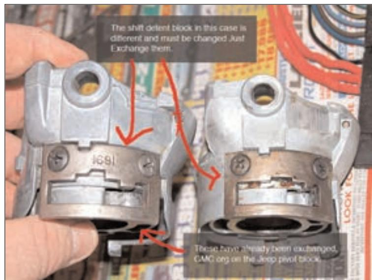
Make sure you lock tight the bolts that hold the lower tilt block in place. Red or green lock tight would not be out of the question.
