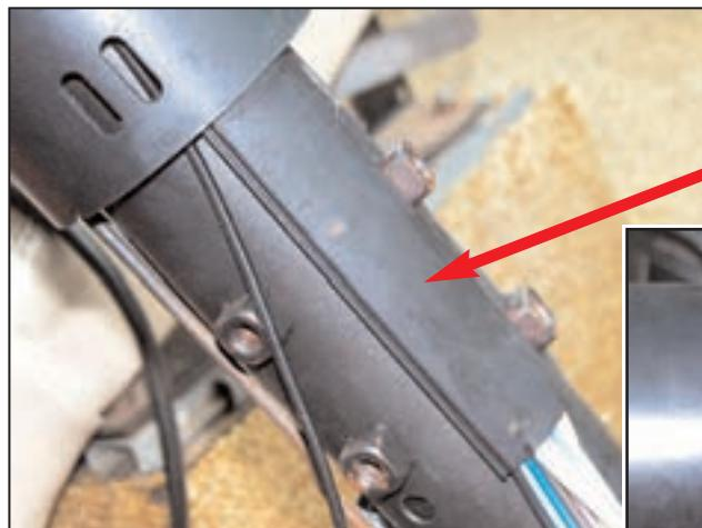
You need to remove the support bracket so the plastic wire loom can be removed.
