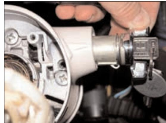
To go any farther you need a lot of extra wire for the blinker switch so the upper cover can be removed. If you are upgrading the column you might as well remove it now. It will make it easier later. This will require you to remove the bracket that holds the upper part of the column in place.
