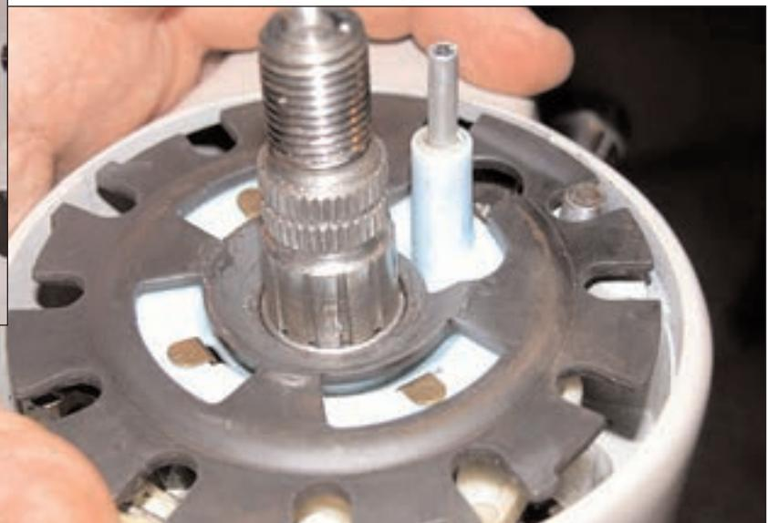
**Put on the levers and the column is back together.**
