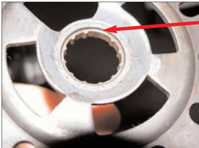
The reverse procedure is used to reinstall the locking plate using the spring compressor.
