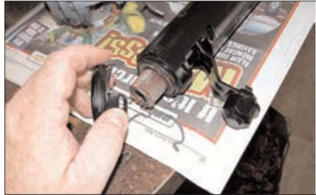
**Grease and install the lower bearing in the upper tilt block. Note that only grease holds these bearings in place**
