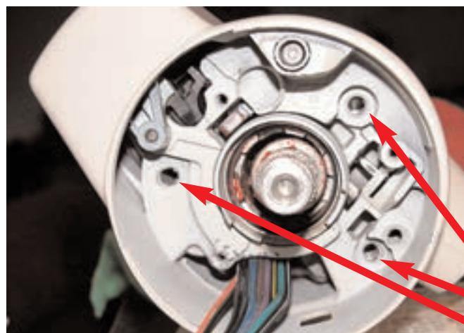
Remove the three screws and slide the cover off
