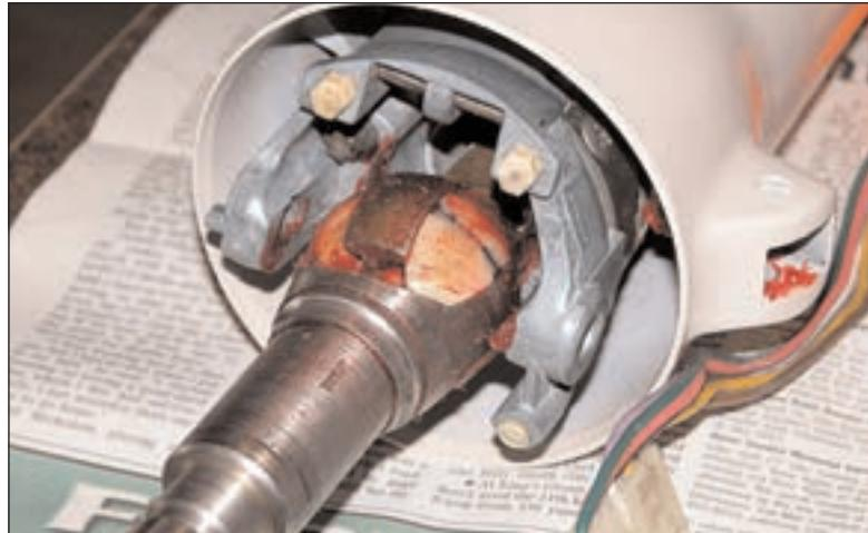
**Replace or repack the lower steering shaft bearing and reinstall the bearing, the cap, and the retainer.**
