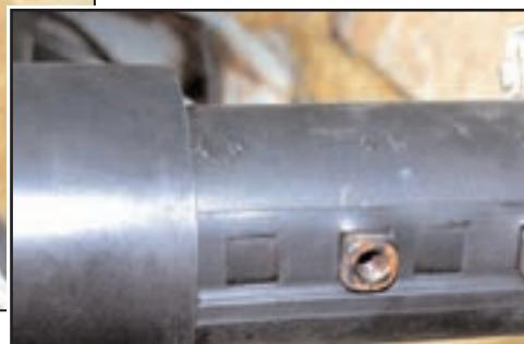
Once you get the bracket off, pull the wire loom off the braze-ons. Then pry the loom open and take it off.
