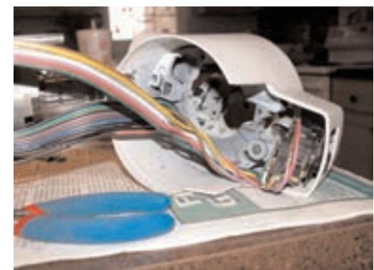
**Put the tilt lever back on and tilt the column to the up position. This takes some of the tension off the spring.**
