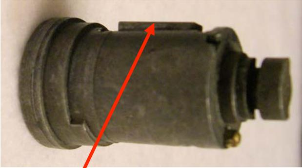
The side bar is out when the key is removed, and the plug will not turn.
