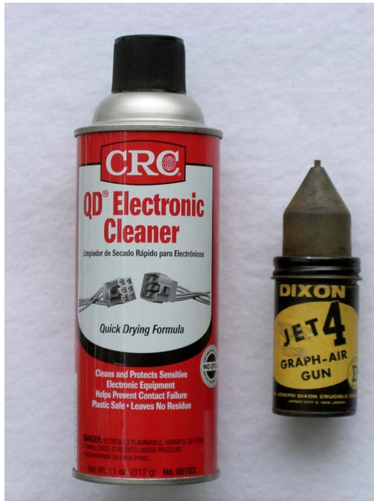
This cleaner dissolves oil and the dirt runs out of the lock. It dries fast and leaves no residue. Use only powdered graphite to lube locks.
