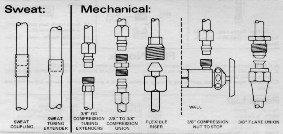
NOTE: We suggest that the 3/8 inch sweat supplies be assembled and soldered before installing the faucet.
