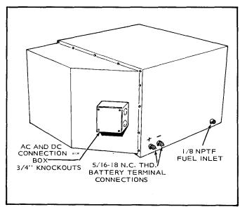
FIGURE 2. EXTERNAL CONNECTIONS
