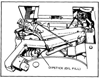
FIGURE 17. DIPSTICK LOCATION (TOP VIEW)
