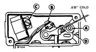
FIGURE 13. BREAKER POINT ADJUSTMENT
