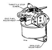
FIGURE 15. CARBURETOR ADJUSTMENTS
