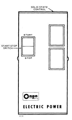
FIGURE 12. PLANT-MOUNTED START-STOP SWITCH
