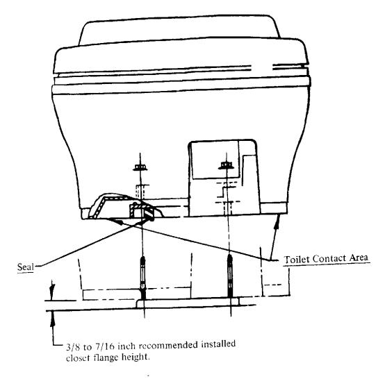
Lay a straight edge across closet flang and measure distance to floor at toilet contact area to check flange installation. Too much gap may cause the flush mechanism to bind. Too little gap may prevent a good seal.
