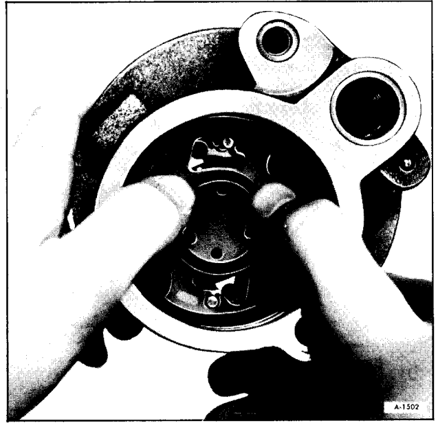
Figure 21—Installing Pressure Plate
