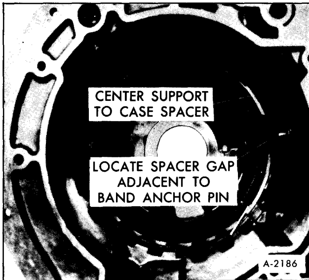
Figure 72—Installing Support-to-Case Spacer
