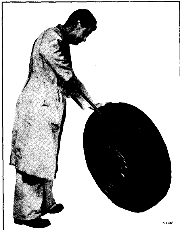
Figure 11—Prying Second Bead from Rim
