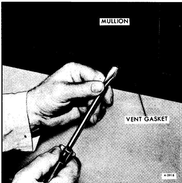
Figure 14—Unseating Vent Gasket
