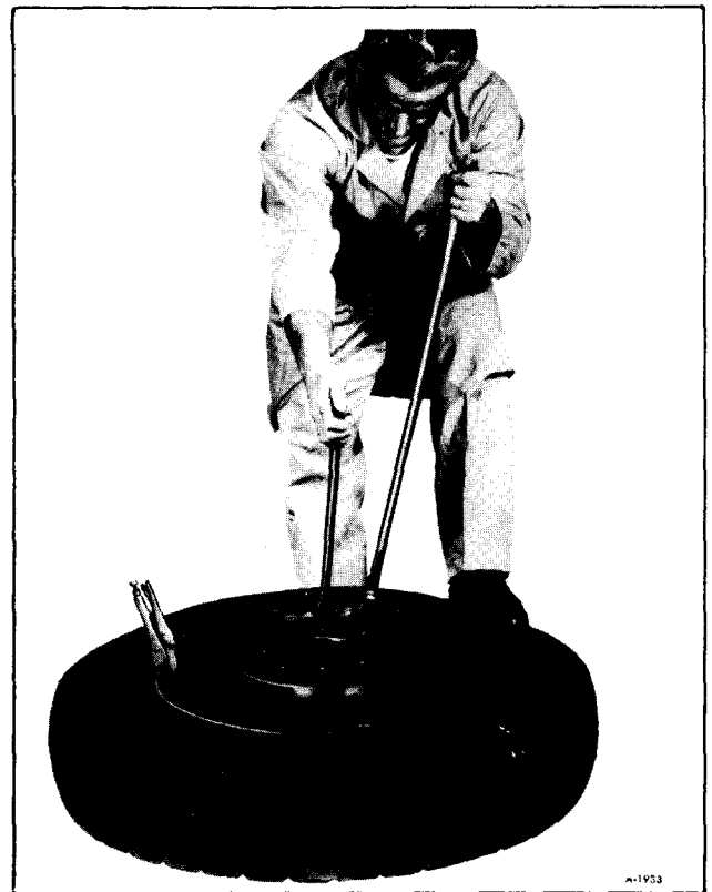
Figure 7—Working Second Bead Onto Rim
