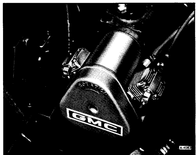
Figure 3—Air Compressor Location (Dana)
