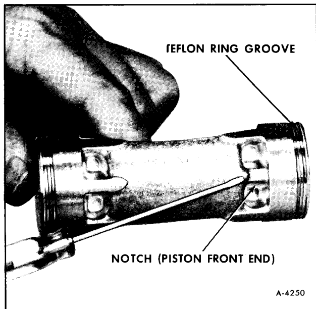
Figure 71—Notch Identifying Front End of Piston
