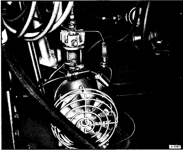
Figure 2—Air Compressor Location (Brown)
