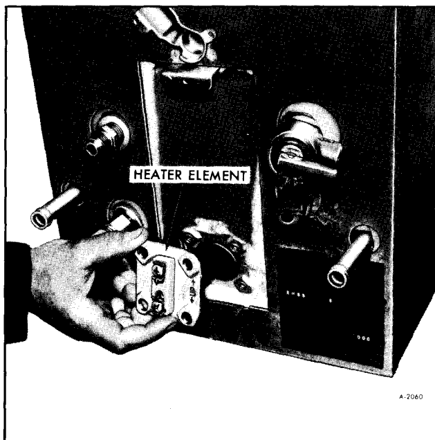
Figure 41—Installing Heater Element
