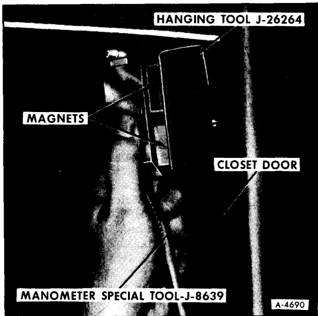
Figure 3—Hanging Manometer
