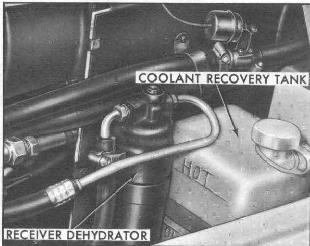
Coolant Recovery Tank (Typical)
