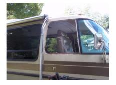
Before I replace the window felt, I decided to mask off and paint the window frame. I used black engine enamel because I had some.
