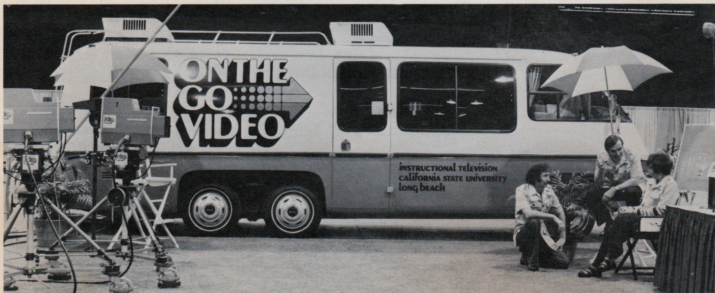
This 26-foot GMC Transmode unit is the mobile control room for "On the Go Video" operations of the Instructional Television department of California State University, Long Beach. The unit transports all needed production equipment and as many as seven staff persons, besides housing a complete control room installation.
