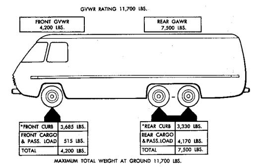
\*Curb weight is the weight of the vehicle without driver, passenger, or cargo, but does include fuel and coolant
