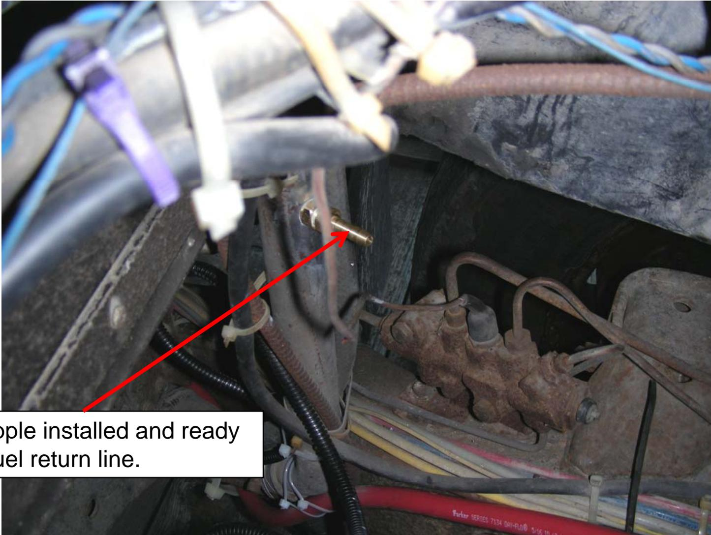
Hose nipple installed and ready for the fuel return line.
