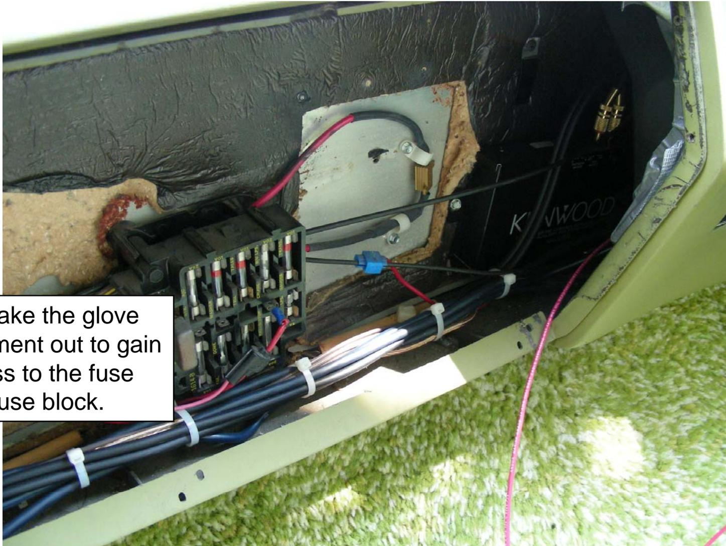
I had to take the glove compartment out to gain full access to the fuse chassis fuse block.
