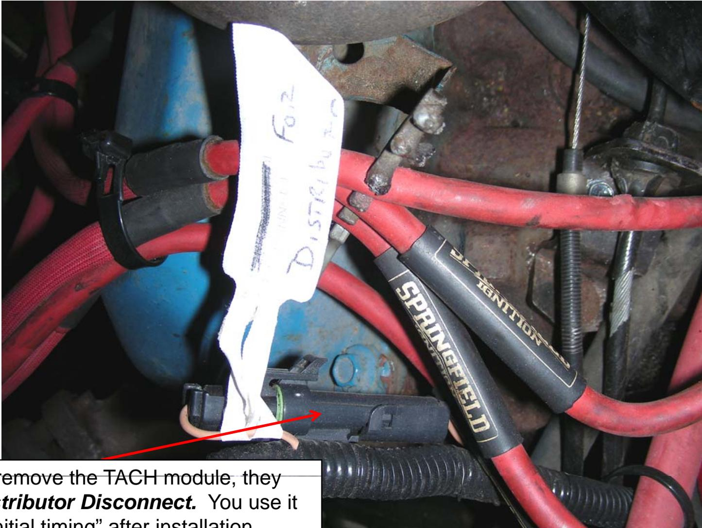
When they remove the TACH module, they add this **Distributor Disconnect**. You use it to set the "initial timing" after installation
