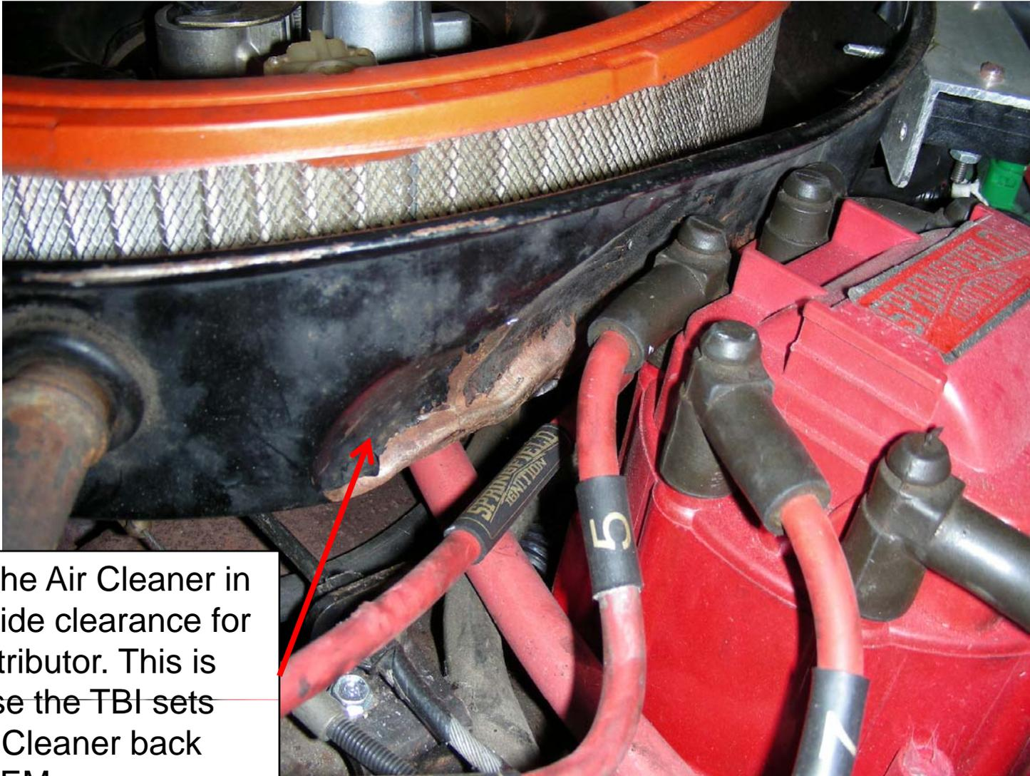
I bent the Air Cleaner in to provide clearance for the distributor. This is because the TBI sets the Air Cleaner back from OEM.
