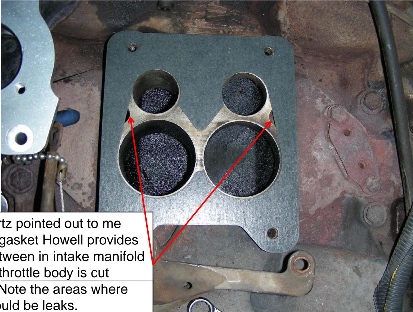
Paul Bartz pointed out to me that the gasket Howell provides to go between in intake manifold and the throttle body is cut wrong. Note the areas where there would be leaks.
