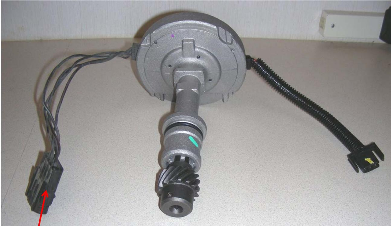
Another view of AutoZone distributor with "the distributor to ECM wiring harness" from the donor installed and ready for the engine.
