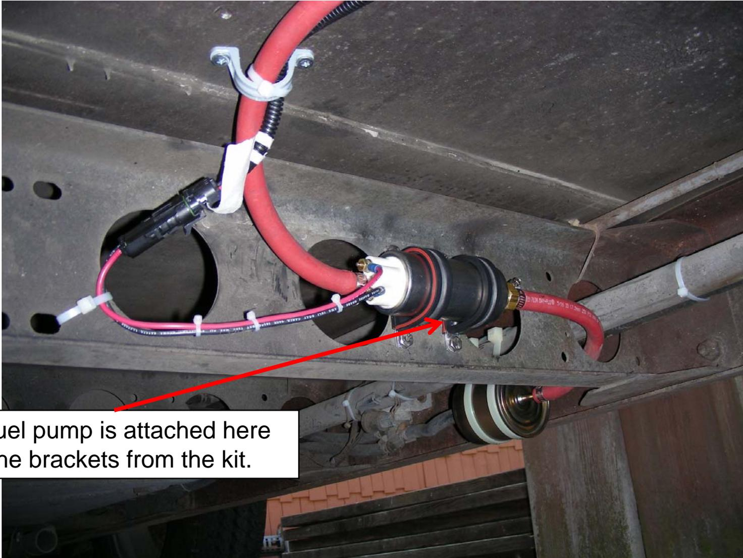
The fuel pump is attached here with the brackets from the kit.
