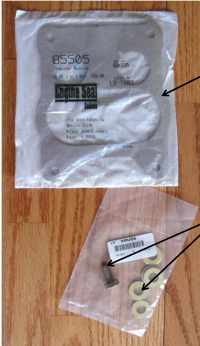
Thick Quadrajet to manifold gasket to replace the thin gasket in Howell's kit.
