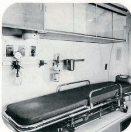
2. One of two Ferno-Washington cots. Two additional stretchers may be suspended from the interior roof.
