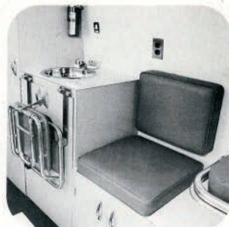
3. Attendant seat at foot of cot, sink and folding "stair chair", one of four electrical outlets and additional cabinet space.
