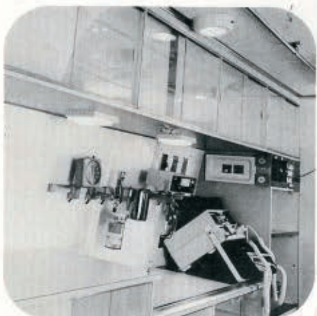
4. Overhead cabinets with sliding, clear plexi-glass doors. Life system monitoring and telemetry units below.
