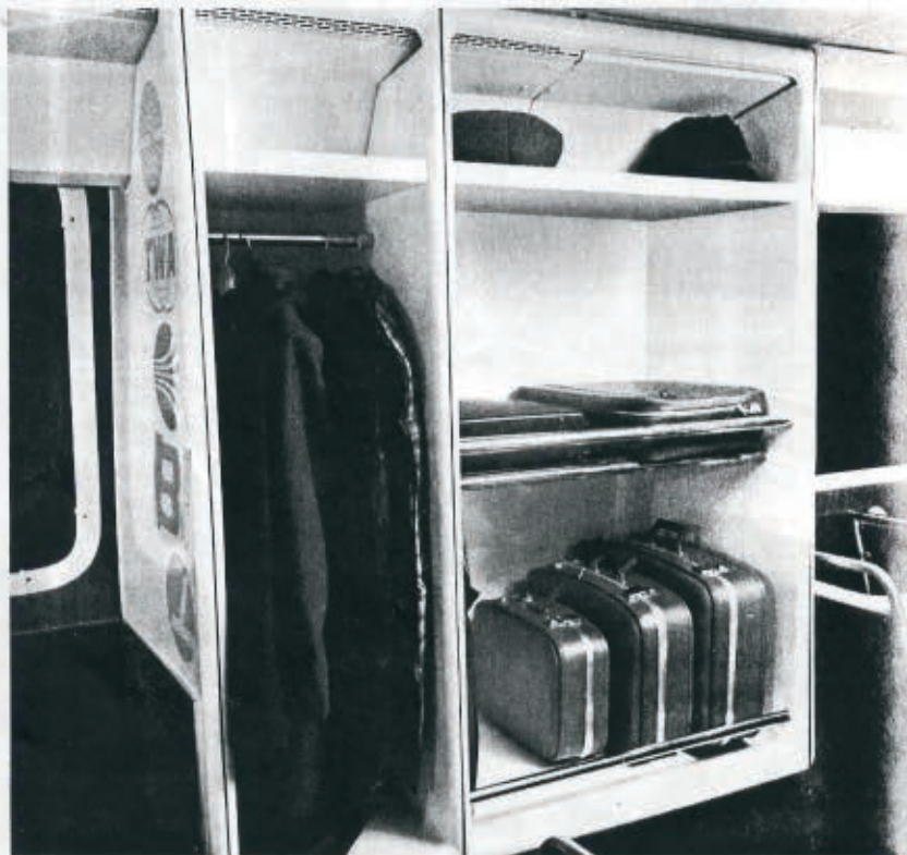
Rear luggage compartment has room for hats, coats, garment bags as well as luggage. This rear luggage module will be 51" wide.
