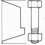
In this full size shank fastener, the maximum load is still limited by the root area of the thread.
