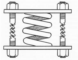
But now the fastener stretch is reduced because of the larger body diameter and this will make the joint less compliant. (Less sense of humor.)
