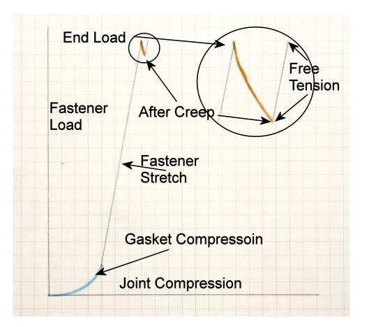
The name of the game with cylinder head gaskets is the ratio of bolt load to fire pressure
