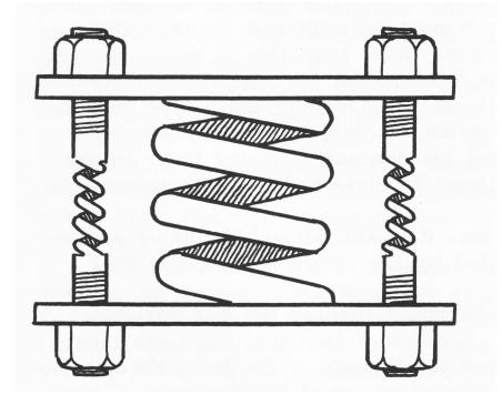
When you torque a fastener, you are imbuing it with tension. You are, in fact, cocking a spring.
