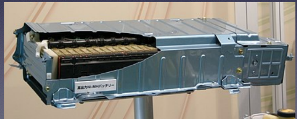
High-power Ni-MH battery of Toyota NHW20 Prius, Japan
