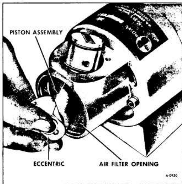
Figure 28—Removing Compressor Piston
