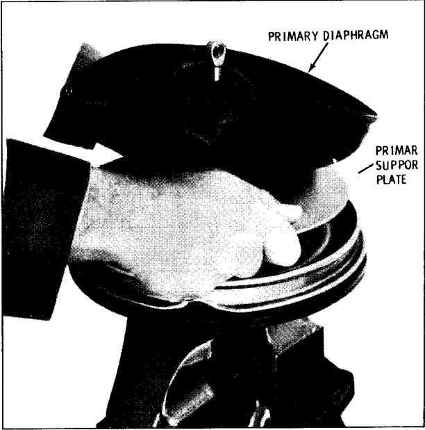
Figure 39—Unlocking Power Piston
