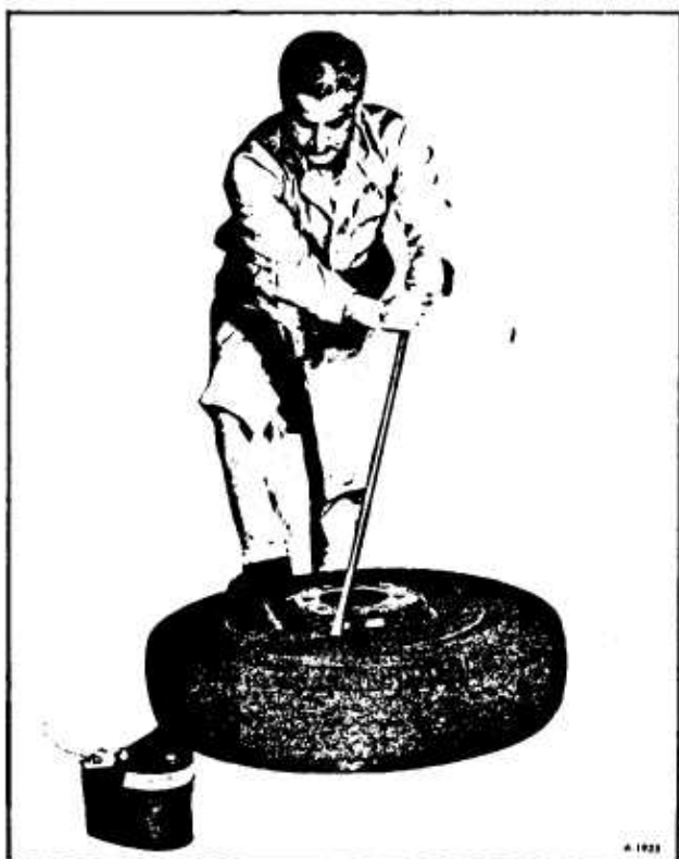
Figure 9—Lifting Bead Over Rim
