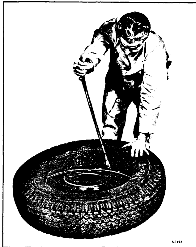
Figure 6—Working Bead Onto Rim
