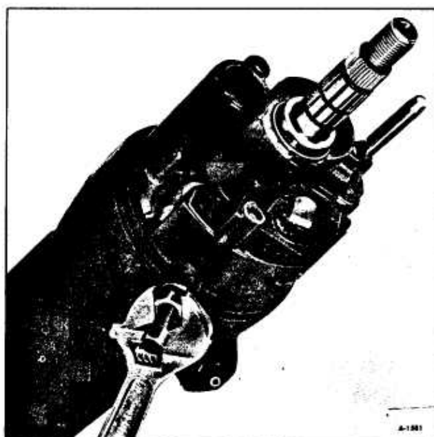
Figure 99—Removing Pivot Pins
