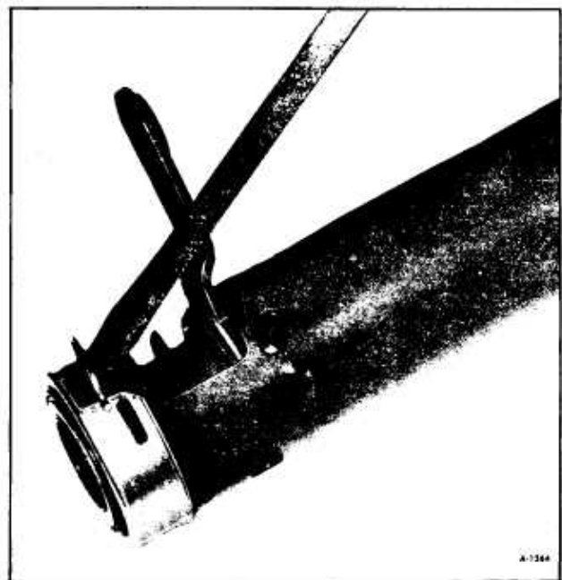
Figure 82—Removing Bearing Adapter Clip
