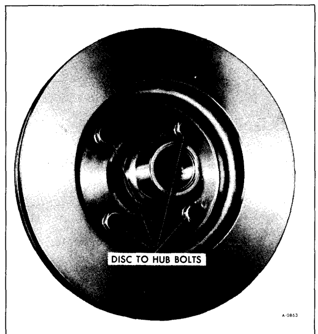
Figure 58—Hub to Disc Bolts
