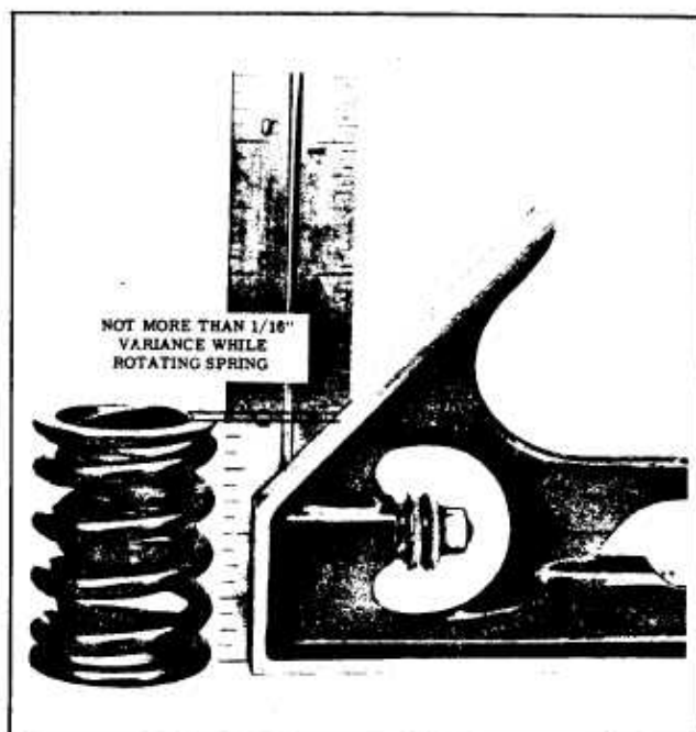
Figure 19-Checking Valve Spring
