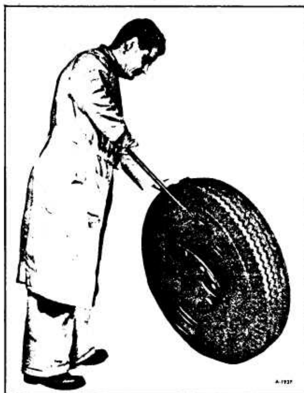
Figure 11—Prying Second Bead from Rim
