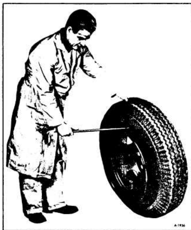
Figure 10—Inserting Tire Iron in Second Bead
