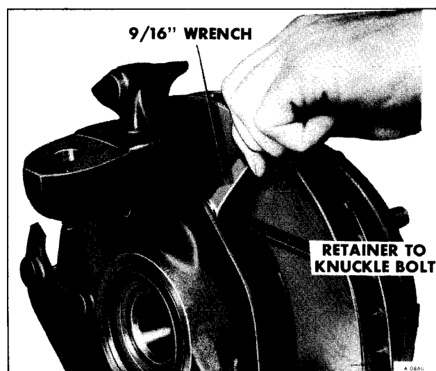
Figure 17—Removing Retainer from Knuckle
