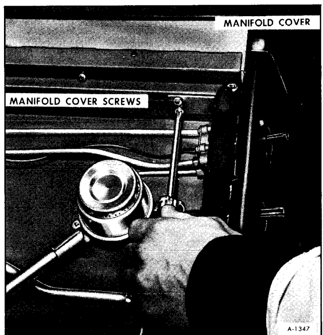
Figure 7-Removing Manifold Cover Screws (Upper)
