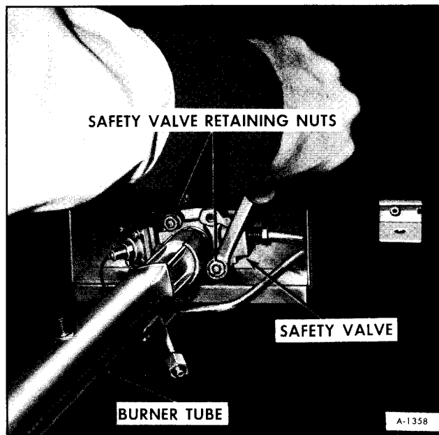
Figure 18-Removing Nuts Holding Safety Valve
