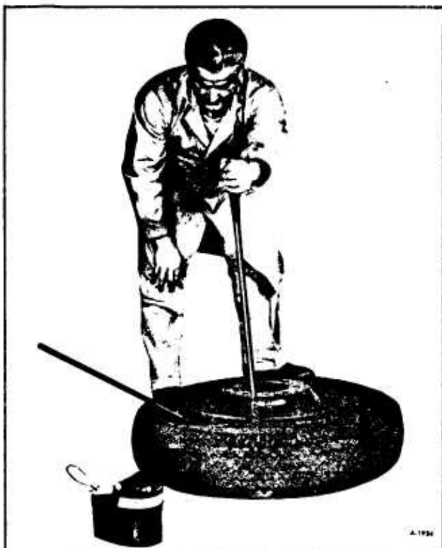
Figure 8—Inserting Tire Iron to Lift Bead
