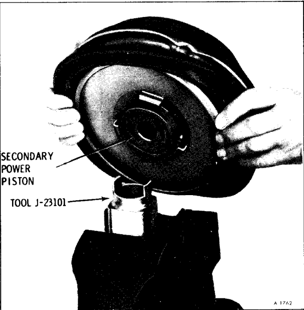
Figure 38—Positioning Secondary Power Piston
