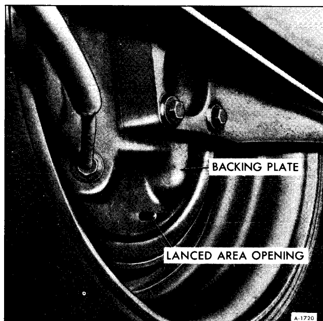
Figure 6-Lanced Area in Backing Plate
