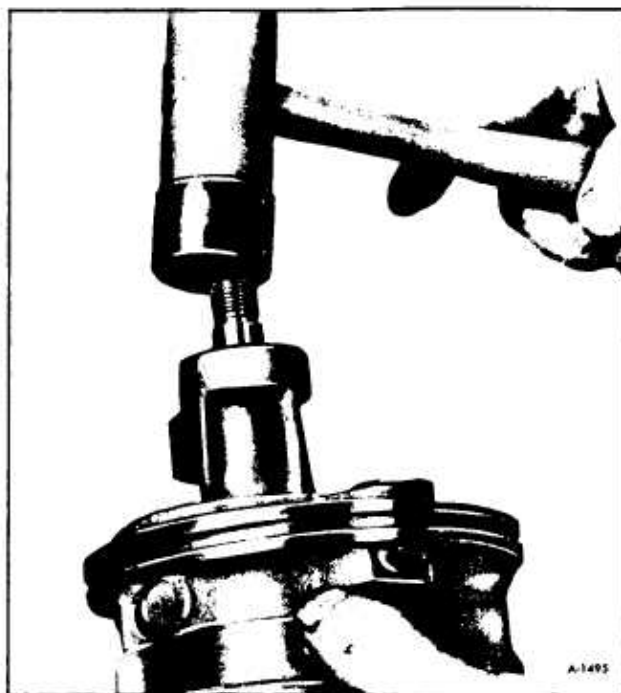
Figure 13—Tapping Shaft to Unseat Pressure Plate
