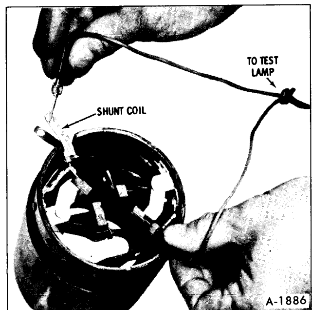
Figure 47-Checking Shunt Field Coil
