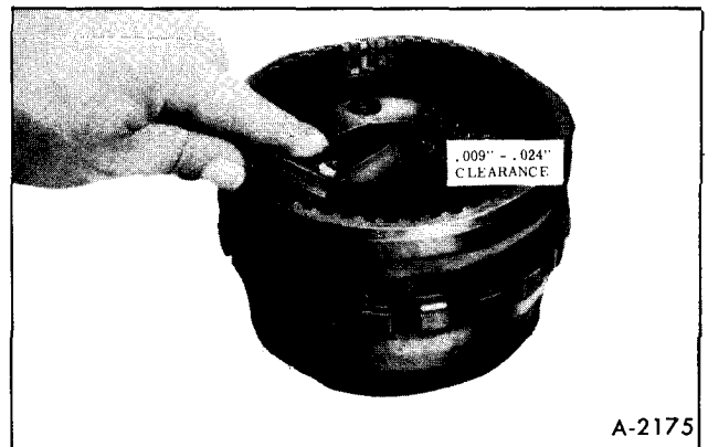
Figure 58—Check-Pinion End Play
