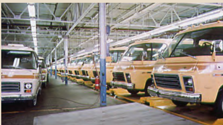
GMC Motorhomes conveyed sideways on dollies along assembly line.
