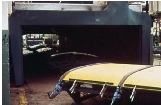
Top roof panel to frame bonding entering cure oven.
